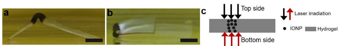
Figure S3. Bending of the composite hydrogel sheet under laser irradiation. (a) The hydrogel sheet bent downwards when laser was irradiated onto the bottom side of the hydrogel (red arrows in (c)); (b) the same sheet bent upwards when laser was irradiated onto the top side of the hydrogel (black arrows in (c)); This side was in contact with agarose stamp during ion diffusion. Scale bars: 3mm.
