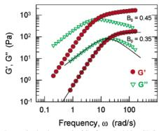
Figure 3. Dynamic rheology at 25 °C of two lecithin-SDC mixtures in cyclohexane. The samples contain 100 mM lecithin and the SDC/lecithin molar ratios,  $B_0 = 0.35$  and 0.45. The plot shows the elastic modulus G'( $\bullet$ ) and the viscous modulus  $G''(\nabla)$  as functions of frequency  $\omega$ . Fits to a single-relaxation-time Maxwell model are shown as solid lines for the  $B_0$ = 0.35 sample.
