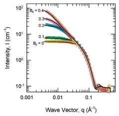
**Figure 6.** SANS data from samples in deuterated cyclohexane containing 20 mM lecithin and different SDC/lecithin molar ratios  $B_0$ . The solid curves through the data are fits to appropriate models (see text for details).
