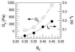
Figure 4. Plateau modulus  $G_p$  and relaxation time  $t_R$  for lecithin-SDC mixtures in cyclohexane as a function of the SDC/lecithin molar ratio  $B_0$ . The lecithin concentration in these samples is 100 mM. The parameters were extracted from dynamic rheological spectra such as those shown in Figure 3.
