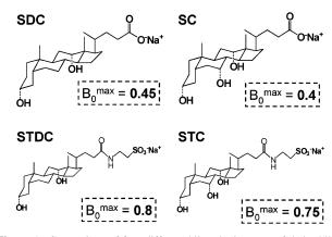
**Figure 8.** Comparison of four different bile salts in terms of their ability to induce viscoelastic reverse micelles of lecithin in cyclohexane. The lecithin concentration is fixed at 100 mM, and  $B_0^{\rm max}$  is the molar ratio of the respective bile salt/lecithin mixture at which the zero-shear viscosity reaches a maximum.
