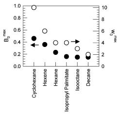
**Figure 7.** Comparison of bile salt (SDC) and water in terms of their ability to induce viscoelastic reverse micelles of lecithin in six different solvents. The lecithin concentration is fixed at 100 mM. The parameters plotted are the molar ratios of bile salt/lecithin ( $B_0^{\rm max}$ ) and water/lecithin ( $w_0^{\rm max}$ ) at which the zero-shear viscosities of the respective mixtures reach a maximum.
