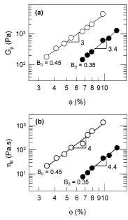
**Figure 5.** Rheological parameters for lecithin—SDC mixtures as a function of the lecithin volume fraction  $\phi$ . Data are provided for two values of the SDC/lecithin molar ratio  $B_0$ . Figure 5a shows the plateau modulus  $G_p$ , and Figure 5b, the zero-shear viscosity  $\eta_0$ .
