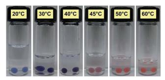
**Fig. 3** Colorimetric response to temperature of PDA vesicle-bearing chitosan–SDBS capsules in a pH 6 buffer solution.
