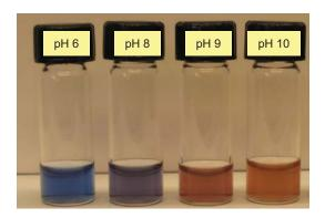
**Figure S1.** UV-Vis spectra (top) and photographs (bottom) of PDA vesicle solutions at different pH. The solutions each contain 0.33 mM of the diacetylenic amphiphile and the solution pH was varied by using phosphate buffers in different proportions.
