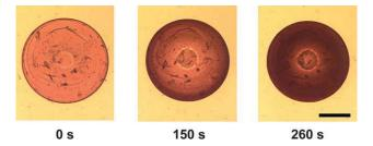
**Fig. 4** Optical micrographs showing the progression of the colorimetric transition in a PDA vesicle-bearing capsule. The capsule is transferred from a pH 6 buffer to a pH 7 buffer at t=0. At this initial stage, the capsule has a blue color and appears bright. With increasing time, a dark front (purple) moves through the capsule. The scale bar represents 1 mm.
