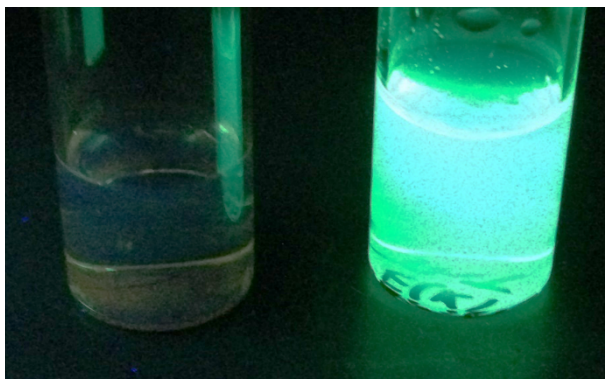
Figure S3. Thioflavin T 6 fluoresces in the presence of the GB hydrogel. While ThT 6 (100 \mu M) is not visibly fluorescent under a UV lamp (left, vial 100 \mu M ThT), when exposed to a 1 wt% K^+ GB hydrogel (36 mM G 1 , 18 mM KB(OH)_4 ) there is a notable fluorescence response (left, vial + GB- K^+ ). This is presumably due to the ability of ThT 6 to dock onto the G_4 -quartets within the GB hydrogel (right).
