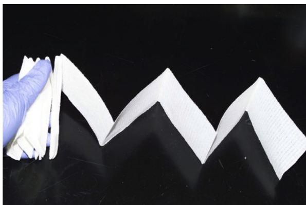
Fig. 1 – Photograph of hm-C gauze. Gauze was aired dried after coating with hm-C solution and then Z-folded for better ease of packing into the wound. (Color version of figure is available online.)
