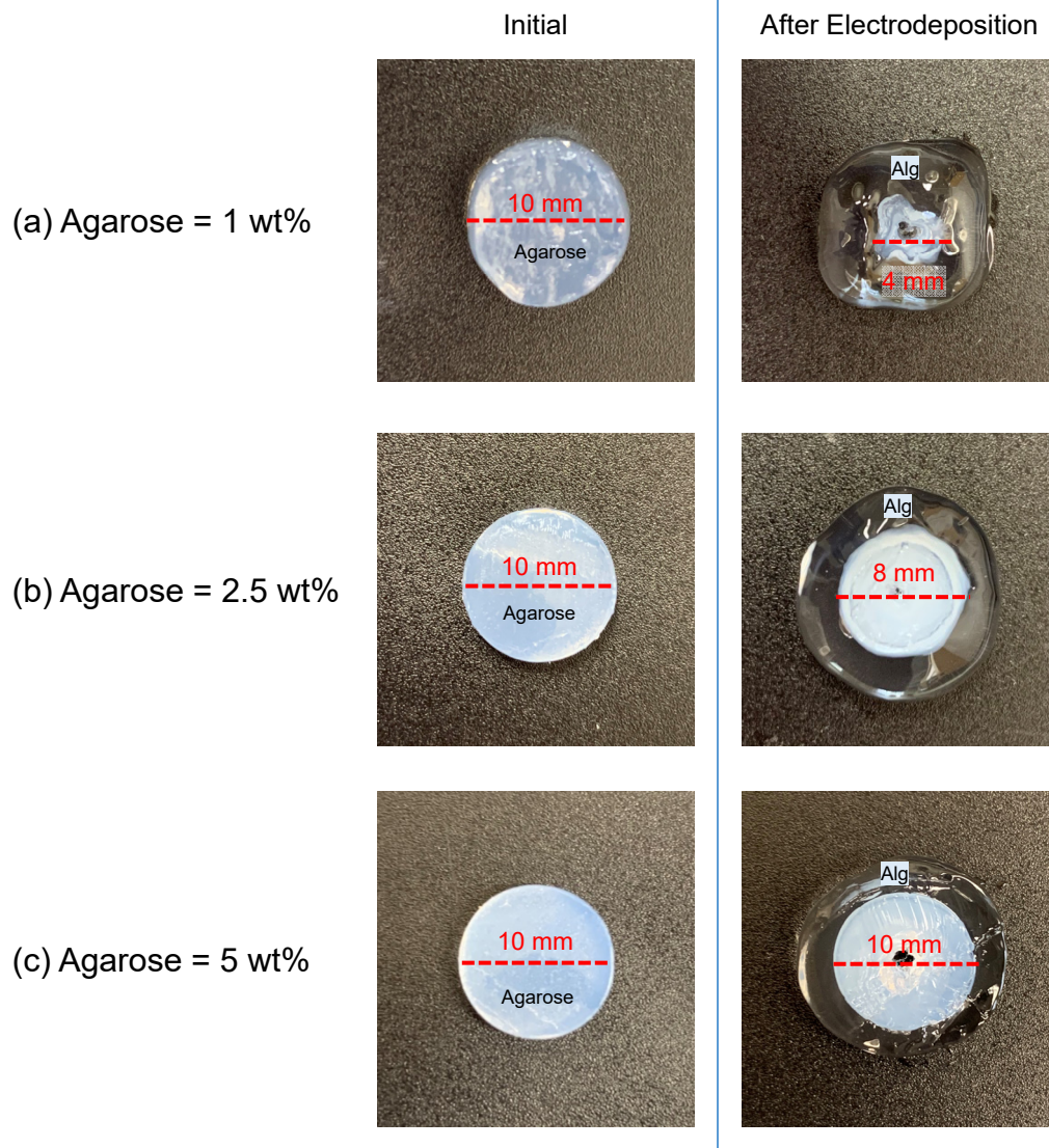
Figure S1. Effect of agarose concentration on the core-shrinking phenomenon observed during electroformation. The agarose core was loaded with 0.01 wt% \text{Ca}^{2+} in each case and placed in a solution of 1 wt% Alg. Electroformation was done at a voltage of 10 V for 5 min, much like in Figure 3. Images are shown at the initial stage (left) and after electrodeposition (right). Note that the clear layer around the core on the right is the Alg gel. The core shrinks in the case of agarose concentrations of (a) 1 wt% and (b) 2.5 wt%, but not in the case of (c) 5 wt%.
