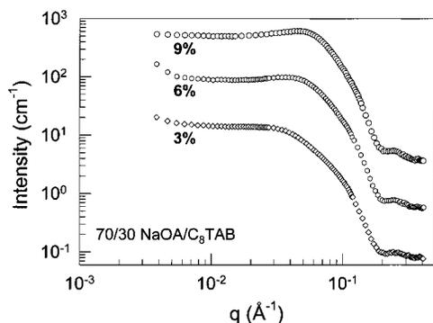
**Figure 10.** SANS spectra for 70/30 NaOA/C<sub>8</sub>TAB solutions in D<sub>2</sub>O at different surfactant concentrations. The data for the 3% sample are absolute values while the remaining curves are offset by factors of 5 for clarity.
