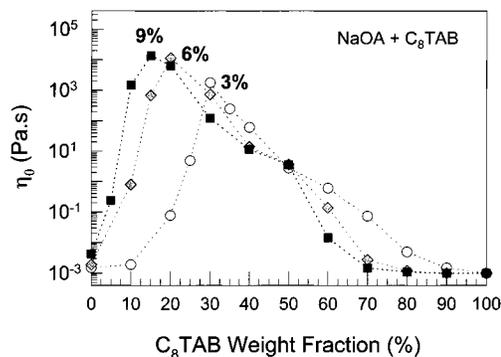
**Figure 5.** Zero-shear viscosity  $\eta_0$  of NaOA/C<sub>8</sub>TAB mixtures as a function of composition for three different surfactant concentrations (3, 6, and 9 wt %).
