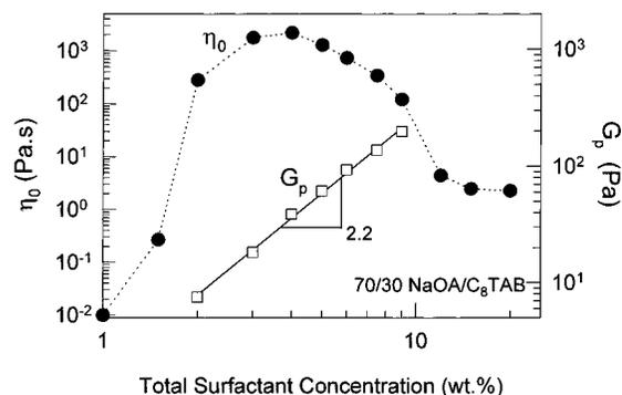
**Figure 4.** Rheology of NaOA/C<sub>8</sub>TAB mixtures as a function of total surfactant concentration. The ratio of NaOA/C<sub>8</sub>TAB is held constant at 70/30. Data for the zero-shear viscosity  $\eta_0$  and the plateau modulus  $G_p$  are shown.
