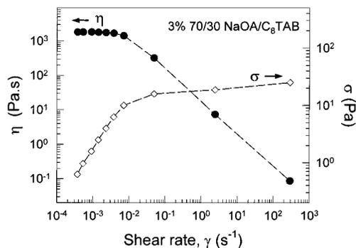
**Figure 3.** Steady-shear rheology of a 3 wt % surfactant solution with the composition 70/30 NaOA/C<sub>8</sub>TAB. The viscosity  $\eta$  and the shear stress  $\sigma$  are plotted as a function of the shear rate.
