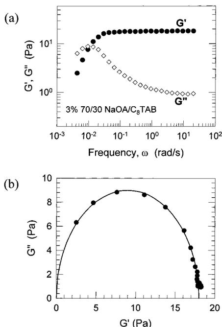
**Figure 2.** Dynamic rheology of a 3 wt % surfactant solution with the composition 70/30 NaOA/C<sub>8</sub>TAB: (a) dynamic frequency spectrum; (b) Cole–Cole plot.
