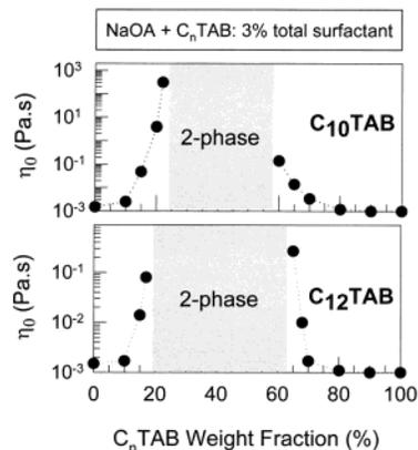
**Figure 8.** Zero-shear viscosity  $\eta_0$  as a function of composition for mixtures of NaOA/C<sub>10</sub>TAB and NaOA/C<sub>12</sub>TAB. The total surfactant content is 3 wt % in all cases. For intermediate compositions in both systems, the samples separate into two (or more) phases.
