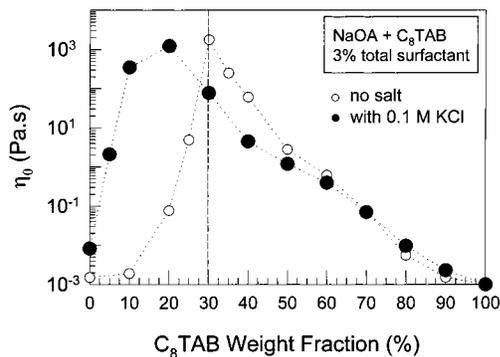
**Figure 6.** Rheology of NaOA/C<sub>8</sub>TAB mixtures in the presence of salt. The zero-shear viscosity  $\eta_0$  is plotted as a function of composition for mixtures containing 0.1 M KCl (filled circles). The data in the absence of salt are also shown for comparison (open circles). The total surfactant content is 3 wt % in all cases.
