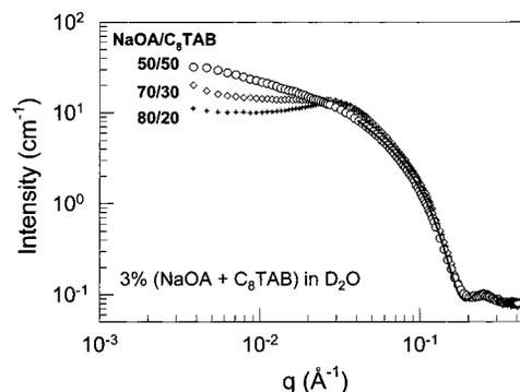
**Figure 9.** SANS spectra for 3 wt % NaOA/C<sub>8</sub>TAB solutions in D<sub>2</sub>O. The solid line is a fit to the 50/50 sample for  $q > 0.04 \text{ \AA}^{-1}$  using a model for monodisperse cylinders. From the fit, a micelle radius of 20 Å is obtained.
