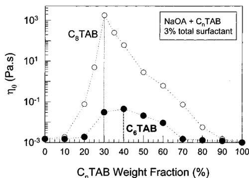
**Figure 7.** Zero-shear viscosity  $\eta_0$  of NaOA/C<sub>6</sub>TAB mixtures as a function of composition. For comparison, data for NaOA/C<sub>8</sub>TAB mixtures are also shown. The total surfactant content is 3 wt % in all cases.
