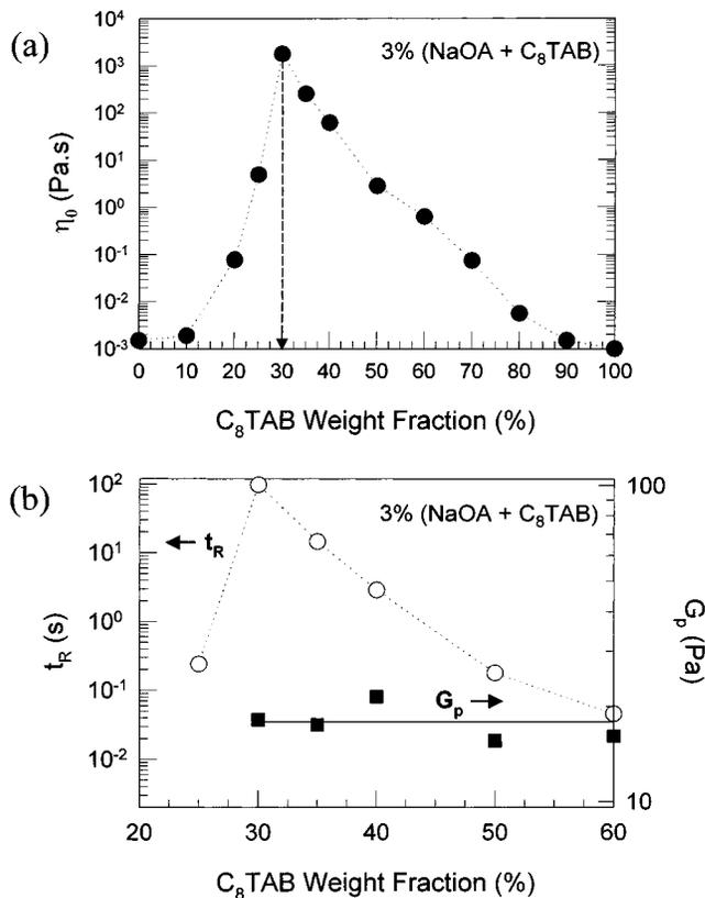
**Figure 1.** Rheology of NaOA/C<sub>8</sub>TAB mixtures as a function of composition for a total surfactant content of 3 wt %: (a) zero-shear viscosity  $\eta_0$ ; (b) relaxation time  $t_R$  and plateau modulus  $G_p$ .
