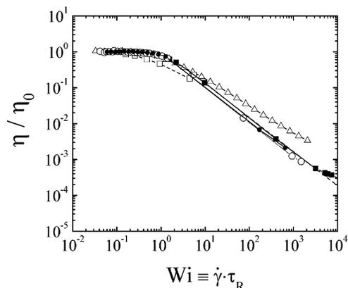
**Figure 3.** Steady-shear rheology for 40 mM EHAC micellar solutions at NaCl concentrations of 60 mM ( $\Delta$ ), 100 mM ( $\square$ ), 600 mM ( $\blacksquare$ ), 800 mM ( $\circ$ ), and 1000 mM ( $\bullet$ ). The sample viscosity is normalized by its zero-shear value and plotted versus the Weissenberg number  $Wi \equiv \dot{\gamma} \cdot \tau_R$ .
