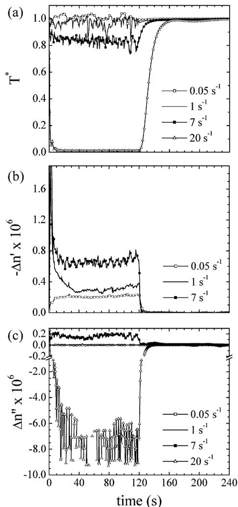
**Figure 4.** Transient rheo-optic experiments on a 40 mM EHAC + 1000 mM NaCl sample in  $\text{H}_2\text{O}$ . The normalized transmittance  $T^*$  (a), the flow-birefringence  $\Delta n'$  (b), and the flow-dichroism  $\Delta n''$  (c) are shown as a function of time during and after shear rates of 0.05, 1, 7, and 20  $\text{s}^{-1}$ . The shear zone is 120 s and is followed by 120 s of relaxation.
