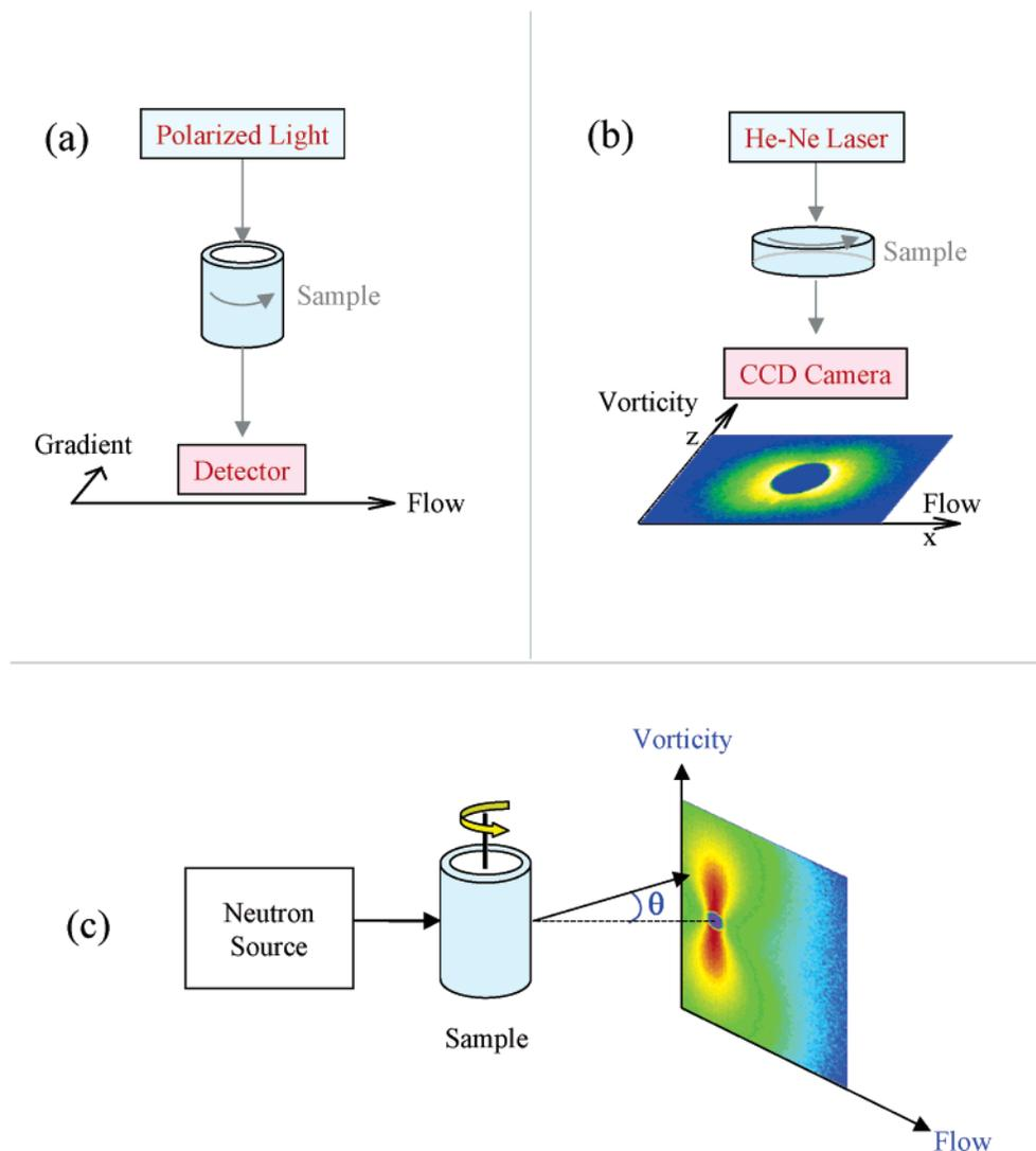
**Figure 1.** Schematic of (a) rheo-optic experiments, (b) flow-SALS experiments, and (c) flow-SANS experiments.
