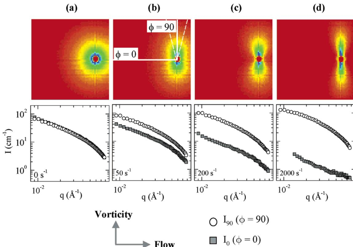
**Figure 6.** 2D flow-SANS patterns at different shear rates for a sample of 40 mM EHAC + 900 mM NaCl in D<sub>2</sub>O. The plots below show the sector-averaged intensity  $I$  about the flow ( $I_0$ ) and vorticity ( $I_{90}$ ) directions extracted from the 2D patterns.
