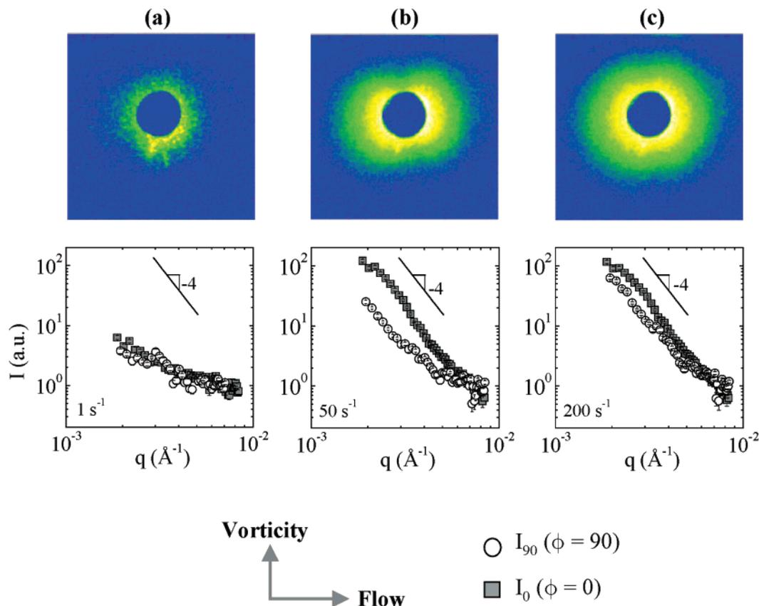
**Figure 8.** 2D flow-SALS patterns for a sample of 40 mM EHAC + 1000 mM NaCl in H<sub>2</sub>O at shear rates of (a) 1 s<sup>-1</sup>, (b) 50 s<sup>-1</sup>, and (c) 200 s<sup>-1</sup>. The plots below show the sector-averaged intensity  $I$  about the flow ( $I_0$ ) and vorticity ( $I_{90}$ ) directions extracted from the 2D patterns.
