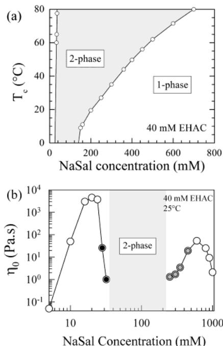
**Figure 10.** Phase behavior and rheology of EHAC/NaSal mixtures at a fixed EHAC content of 40 mM (ref 28): (a) coexistence temperature  $T_c$  vs salt concentration; (b) zero-shear viscosity  $\eta_0$  at 25 °C vs salt concentration. The filled circles in panel (b) denote samples that show shear-induced turbidity.
