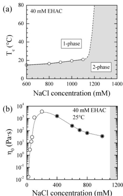
**Figure 2.** Phase behavior and rheology of EHAC/NaCl mixtures at a fixed EHAC content of 40 mM (ref 28): (a) coexistence temperature  $T_c$  vs salt concentration; (b) zero-shear viscosity  $\eta_0$  at 25 °C vs salt concentration. The filled circles in panel b denote samples that show shear-induced turbidity.
