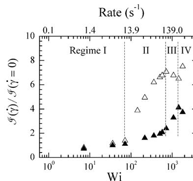
**Figure 9.** Integrated flow-SALS intensities along the flow  $\mathcal{J}_x$  ( $\Delta$ ) and vorticity  $\mathcal{J}_z$  ( $\blacktriangle$ ) directions as a function of Weissenberg number for the 40 mM EHAC + 1000 mM NaCl sample.
