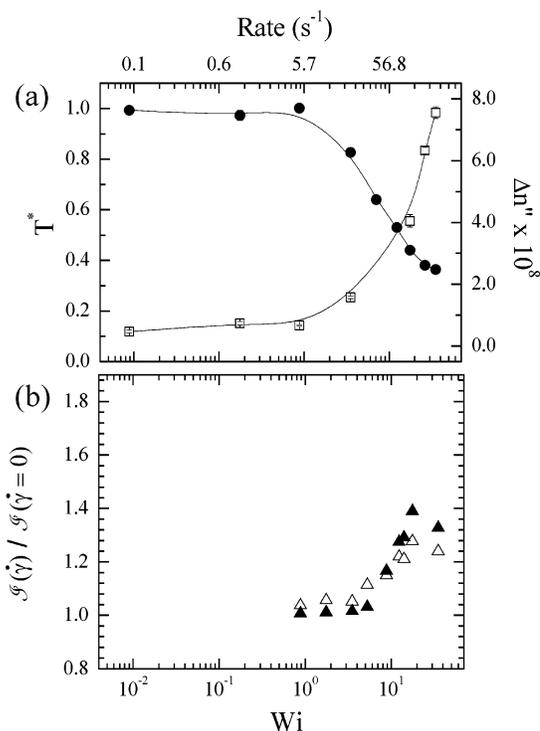
**Figure 11.** Rheo-optic and flow-SALS experiments on a 40 mM EHAC + 250 mM NaSal sample. (a) Steady-state values of  $T^*$  (●) and  $\Delta n''$  (□) as a function of the Weissenberg number. (b) Integrated flow-SALS intensities along the flow  $J_x$  (△) and vorticity  $J_z$  (▲) directions as a function of the Weissenberg number.
