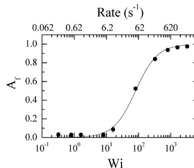
**Figure 7.** Alignment factor based on the flow-SANS sector-averaged data (see text) for the 40 mM EHAC + 900 mM NaCl sample in D<sub>2</sub>O as a function of the Weissenberg number. The line is a fit to the data using eq 6.
