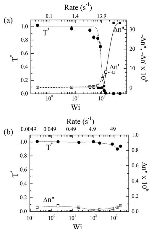
**Figure 5.** (a) Steady-state values of  $T^*$  (●),  $\Delta n'$  (■), and  $\Delta n''$  (□) as a function of Weissenberg number  $Wi$  for a 40 mM EHAC + 1000 mM NaCl micellar solution. (b) Steady-state values of  $T^*$  (●) and  $\Delta n''$  (□) as a function of  $Wi$  for 40 mM EHAC + 60 mM NaCl. The corresponding shear rates are shown for reference on each plot.
