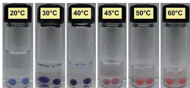
**Fig. 3** Colorimetric response to temperature of PDA vesicle-bearing chitosan–SDBS capsules in a pH 6 buffer solution.
