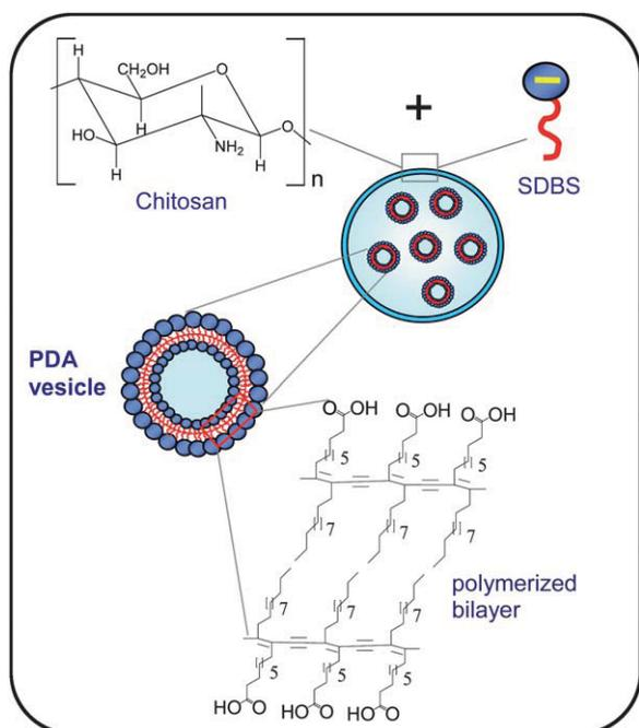
Fig. 1 Encapsulation of PDA vesicles in chitosan–SDBS capsules.
