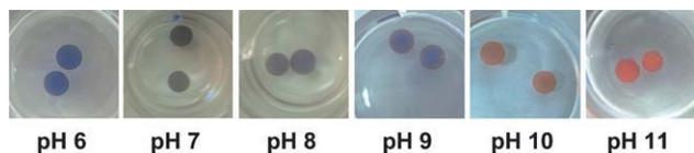
**Fig. 2** Colorimetric response to pH of PDA vesicle-bearing chitosan–SDBS capsules at ambient temperature.
