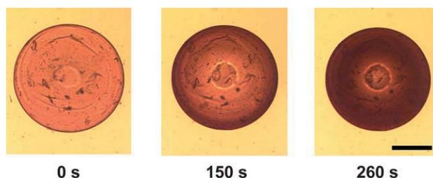
**Fig. 4** Optical micrographs showing the progression of the colorimetric transition in a PDA vesicle-bearing capsule. The capsule is transferred from a pH 6 buffer to a pH 7 buffer at  $t = 0$ . At this initial stage, the capsule has a blue color and appears bright. With increasing time, a dark front (purple) moves through the capsule. The scale bar represents 1 mm.
